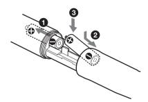
**3** Turn the grip in the direction opposite to the arrow in step 1 to close the battery compartment.
